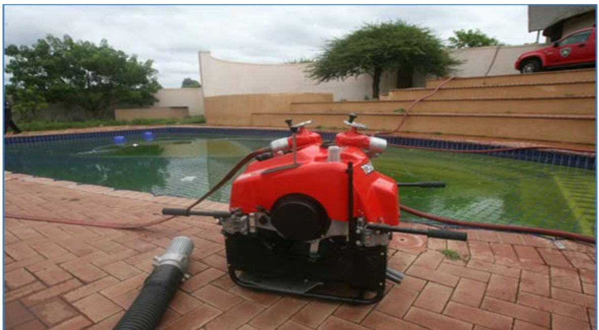
Figure 2: Fire pool/ swimming pool use for fire fighting
