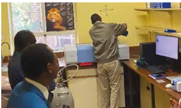
Demonstrating the mobile and high-throughput near-infrared soil spectrometry laboratory machinery
