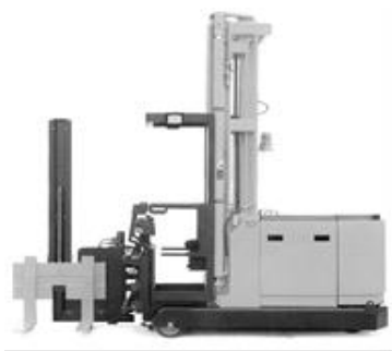
CODE F13 VNA Lift Truck Non-Elevating Cab Services all levels
