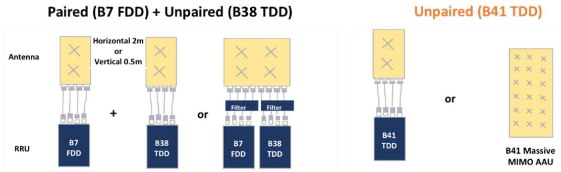
Figure 34: Comparison of FDD and TDD Deployment
