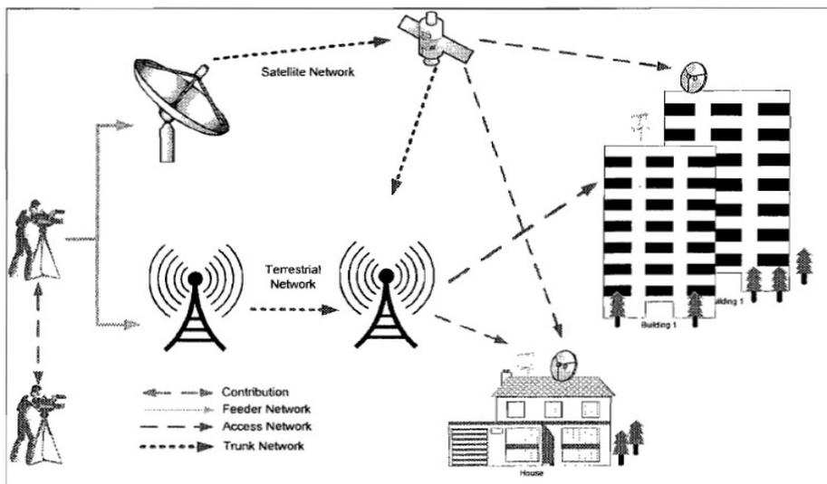
Figure 1: Schematic Presentation of the Infrastructure for Broadcasting Transmission in South Africa.
