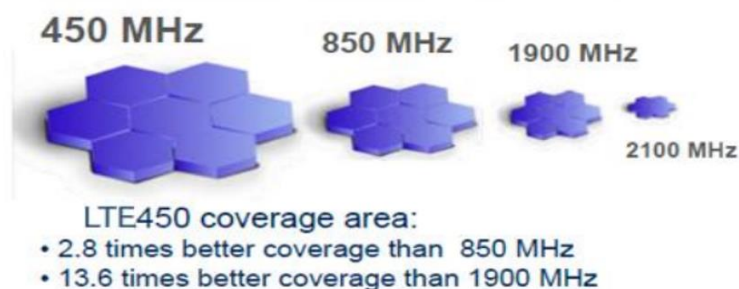
Figure 1: Indicative coverage comparison between different spectrum bands used for wireless communications 19
