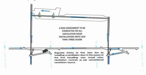
Install ventilation door set in drive between raise lines and regulate air distribution with a brattice set to ventilate the **u-tube**. Management of water control is critical.
