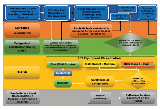
Figure 2: Conformity Assessment Framework for Equipment Authorization
