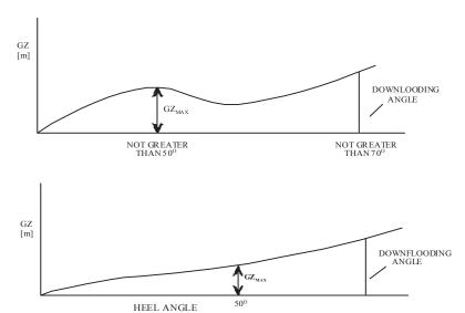
(a) The value of maximum GZ shall be taken at the angle of heel corresponding to the first peak or at 50°, whichever angle is less.
