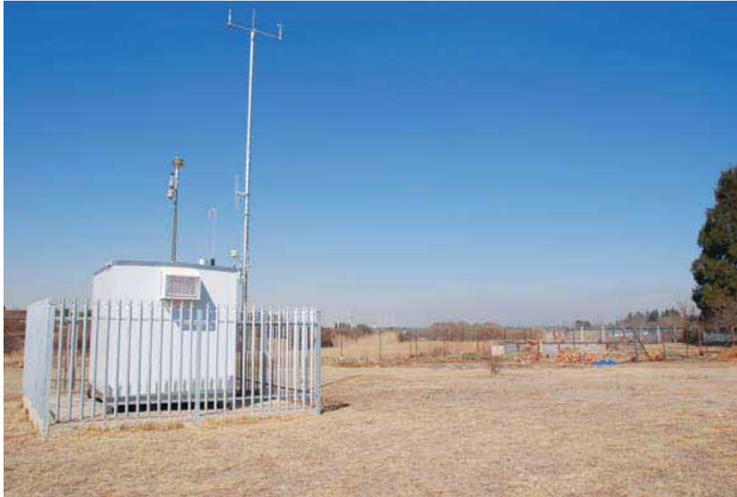
An ambient air quality monitoring station measuring pollution concentrations in Vereeniging.
