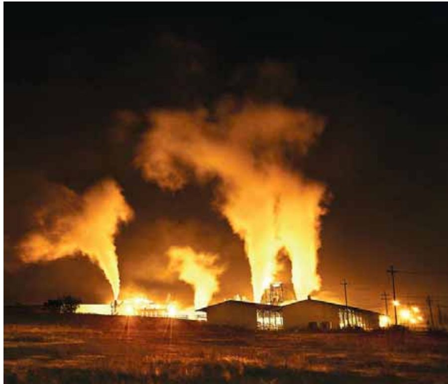
Flaring, to burn off excess gas, is common practice in the industrial sector.
