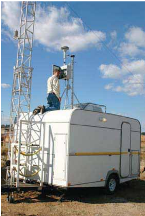
A mobile air quality monitoring station, used most often for once-off research campaigns.
