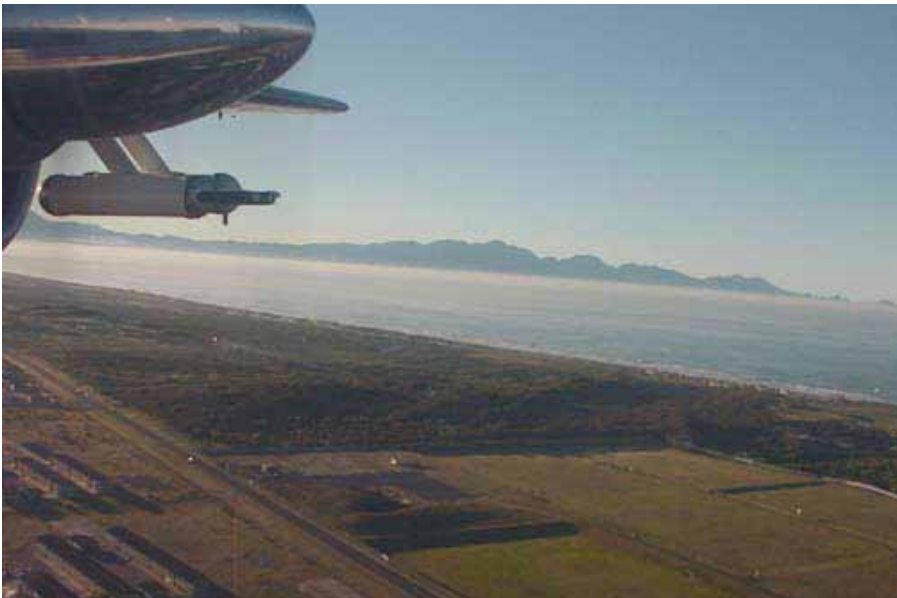
Pollutant concentrations in Cape Town, contributing to the Brown Haze, are measured using instruments fitted to an aeroplane.
