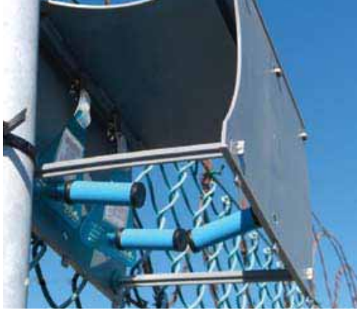
Passive diffusive samplers are used for monitoring air pollution concentrations.
