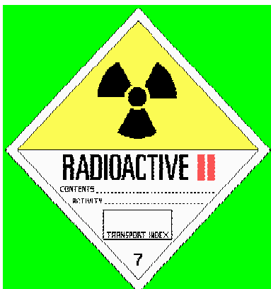
Fig 25: Labels used in packages with radioactive contents
