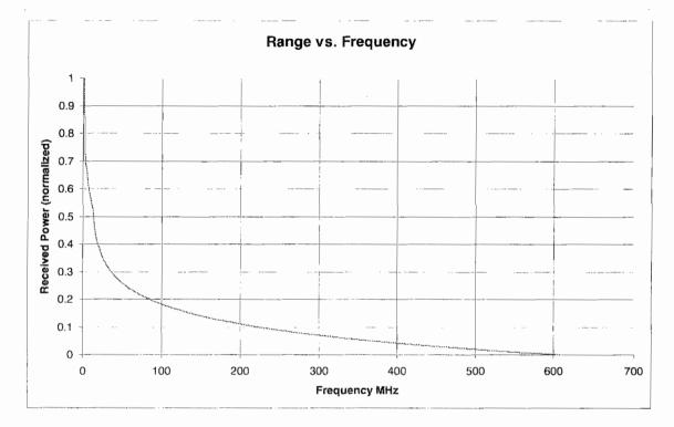
Assuming a transmit power reference and a static distance, different frequencies will result in different path losses from which the received signal levels can be derived.
