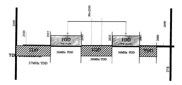
Sentech has an assignment of **50MHz** in the band and WBS has **14MHz**. This leaves a total of **126MHz** spectrum available for further assignments. There are a number of tests currently conducted by different entities under temporary licences.
