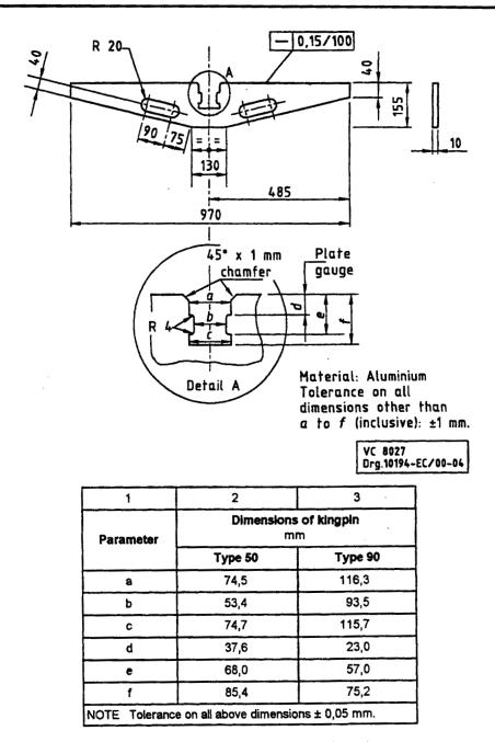
Figure 2 — Details of the kingpin/mounting plate gauge
